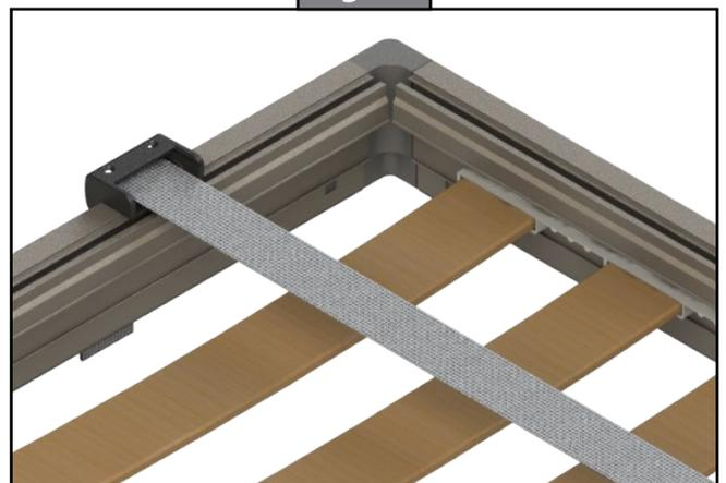
3. Locate the belt mounting assembly (Fig. 20). Unscrew the nuts (Fig. 21C) and slide the belt plates (Fig. 21B) off the belt bracket (Fig. 21A) and set aside. Do this for all four belt brackets.
